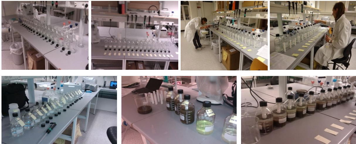
Figure 4 Description of the systematic test procedure for preparing test mixtures with varying concentrations of heat transfer fluid from district heating distribution networks.
