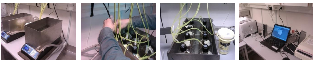
Figure 5 Setup of batch respirometer and connection of pressure regulated aeration device for oxygen input and computer used to measure the input.
