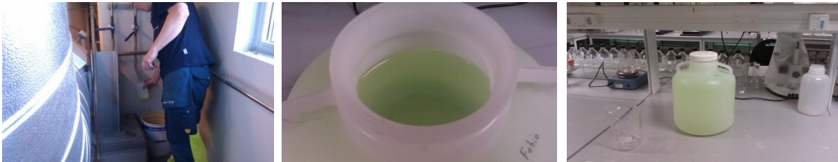
Figure 1 Description of the sampling procedure for heat transfer fluid from the primary distribution network in Kalmar, Sweden.
